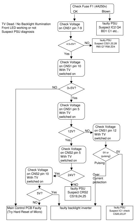
This should only be used as a guide to faultfinding. I do not accept liability for any inaccuracies. This guide is produced solely by loudi out of desperation as info on this PCB is non existent - I am just sharing my own findings/ research :@)
